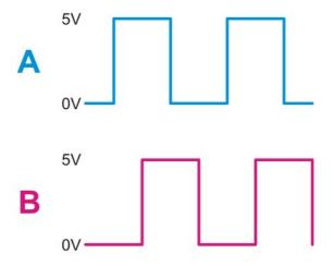
If you only wish to monitor the speed of rotation then you can use either output and simply measure the frequency. The reason for having two outputs is that you can also determine the direction of shaft rotation by looking at the pattern of binary numbers generated by the two outputs. Depending on the direction of rotation you will get either:
